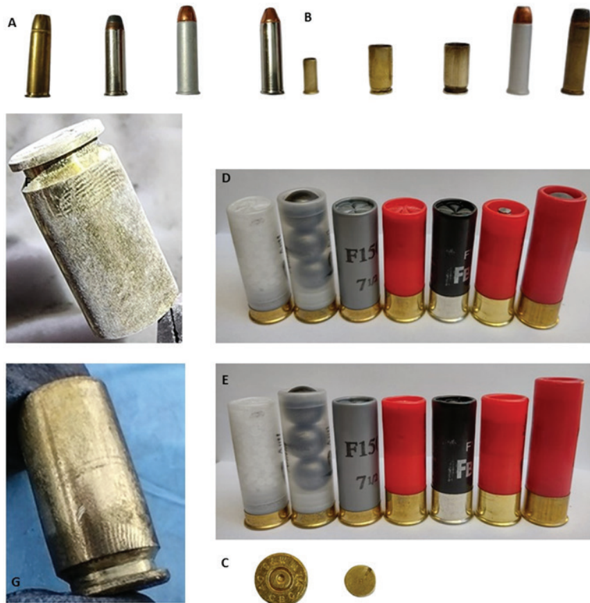
Figure 1. A) Varieties of metal cases (from left to right): brass, stainless steel, aluminum and nickel-plated brass; B) Varieties of breeches, in order: salient breeches with circular flare, two cases of breeches without ribs, salient breeches with central flare and semi-protruding breeches; C) Examples of fuse marks, the first being a central fire and the second a circular fire; D) Top view of varied cartridges, in order: anti-riot, elastomer, bullets for sports practice, SG bullets for defense, SG bullets for defense with nickel-plated base, knock down bullet and knock M3 plus; E) Front view of cartridges; F) Fired cartridge case with latent fingerprint revealed by white developer powder; G) Fired cartridge case with latent fingerprint revealed by black developer powder. Source: own authorship.
